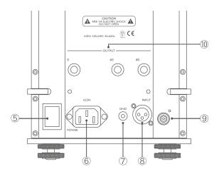
The safety ground of this unit is connected with the ground terminal of the AC cord. Please use an outlet with a ground wire connected. Failure to ground the unit may result in electric shock.
