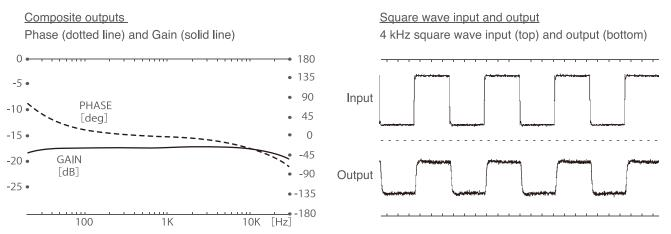
Phase changes in the low and high frequency range are due to the input and output transformers.
